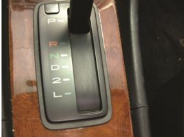
FIGURE 4.9 The gear selector is often called the "PRNDL," pronounced "prindle," regardless of the actual letters or numbers used.
