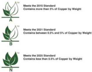
FIGURE 4.11 All boxes of brake linings and pads should be labeled with the leaf mark, which gives a visual clue as to the standard under which the brake friction materials meet certain state laws regarding the amount of copper.
