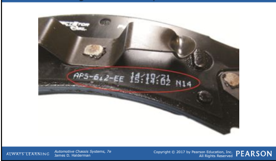
FIGURE 4.13 The “edge codes” are now printed on the backing of the brake pad because there is so much required information that it often does not fit on the edge of the brake pad or shoe.
