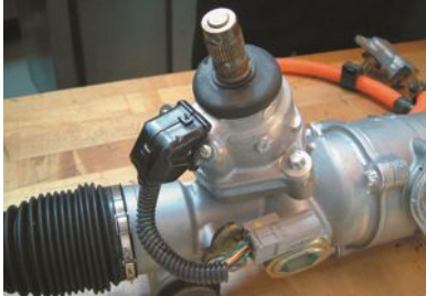
FIGURE 31.3 A Toyota Prius EPS assembly (Courtesy of Tony Martin).
