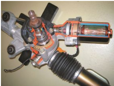
FIGURE 31.2 Honda electric power steering unit cutaway, which is an example of pinion-mounted electric power steering system.
