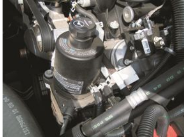
FIGURE 31.9 An electro-hydraulic power steering assembly on a Chevrolet hybrid pickup truck.
