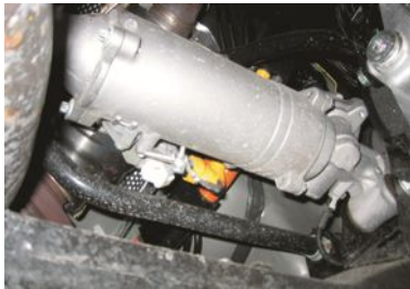
FIGURE 31.1 A rack mounted electric power steering gear on a Lexus RX 400 h taken from underneath the vehicle.
