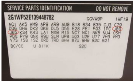
FIGURE 3.9 A typical Service Parts Identification (RPO) sticker is located on the inside of the trunk lid of a GM vehicle.
