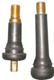
FIGURE 22.7 A conventional valve stem is on the right compared with a rubber TPMS sensor stem on the left. Notice the tapered and larger brass stem.
