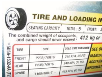
FIGURE 22.1 The tire-pressure placard (sticker) on the driver's side door or door jamb indicates the specified tire pressure.
