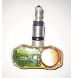
FIGURE 22.6 A clear plastic valve-stem tire-pressure monitoring sensor, showing the round battery on the right and the electronic sensor and transistor circuits on the left.
