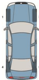
FIGURE 22.17 The sensor relearn procedure is performed in the following order after the system has been placed in learn mode: LF, RF, RR, and then LR.
