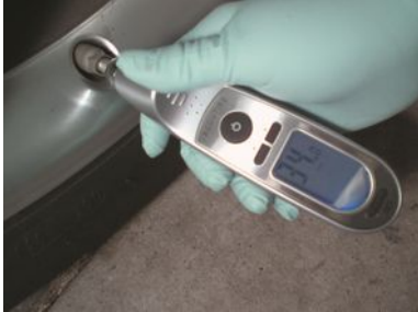
FIGURE 22.18 Always use an accurate, known-good tire-pressure gauge. Digital gauges are usually more accurate than mechanical gauges.
