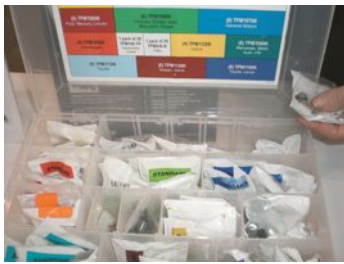
FIGURE 22.20 An assortment of service parts that include all of the parts needed to service a stem-mounted TPMS sensor being installed after removal for a tire replacement or repair.
