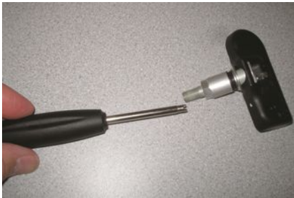
FIGURE 22.19 A clicker-type valve core tool ensures that the valve core is tightened to factory specifications.
