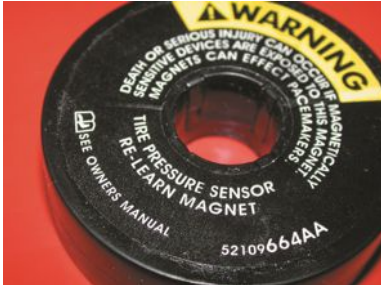
FIGURE 22.15 A magnet is placed around the valve stem to reprogram some stem-mounted tire-pressure sensors.
