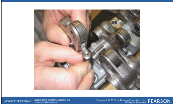
FIGURE 20.11 This Honda valve train photo shows the small spring used to absorb the motion of the rocker arm when the cam is switched to a lobe that has zero lift.
