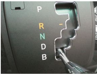
FIGURE 20.8 The “B” position on the shift display on this Lexus RX 400h means braking. This shifter position can be selected when descending long hills or grades.
