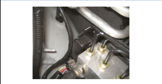
FIGURE 20.13 When working on the brakes on a Ford Escape or Mercury Mariner hybrid vehicle, disconnect the black electrical connector on the ABS hydraulic control unit located on the passenger side under the hood.
