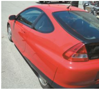
FIGURE 20.1 This Honda Insight hybrid electric vehicle is constructed mostly of aluminum to save weight.
