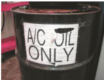
FIGURE 2.10 Air-conditioning refrigerant oil must be kept separated from other oils because it contains traces of refrigerant and must be treated as hazardous waste.
