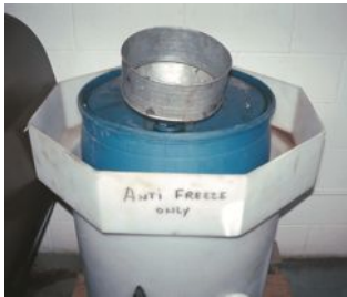
FIGURE 2.8 Used antifreeze coolant should be kept separate and stored in a leakproof container until it can be recycled or disposed of according to federal, state, and local laws.
