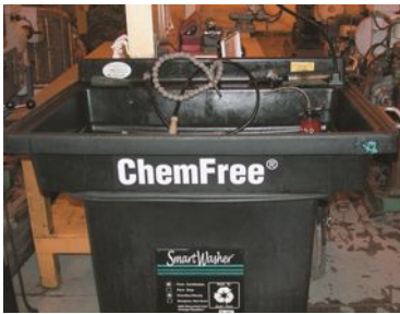
FIGURE 2.7 Using a water-based cleaning system helps reduce the hazards from using strong chemicals.
