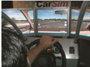
FIGURE 19.3 Using a simulator is the most cost-effective way for vehicle and aftermarket suspension manufacturers to check that the vehicle is able to perform within the FMVSS No. 126 standard for vehicle stability.
