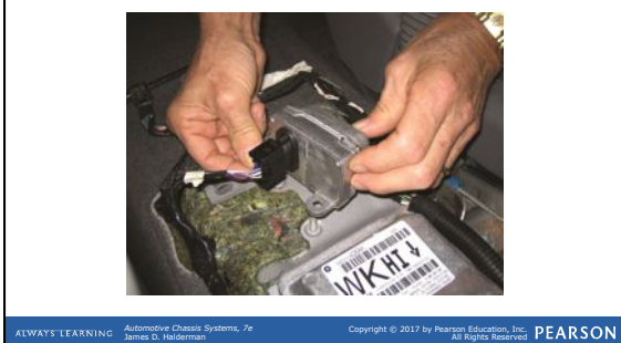
FIGURE 19.8 A lateral acceleration sensor is usually located under the center console and can be easily checked by unbolting it and turning it on its side while monitoring the sensor value using a scan tool.
