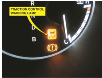
FIGURE 19.12 A traction control or low traction light on the dash is confusing to many drivers.
