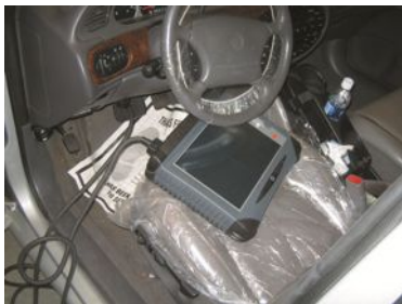
FIGURE 19.13 The use of a factory scan tool is often needed to diagnose the ESC system.
