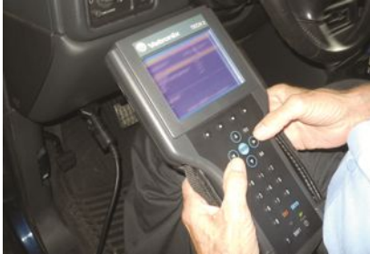
FIGURE 18.6 A Tech 2 scan tool being used to diagnose an ABS problem on a General Motors' vehicle.
