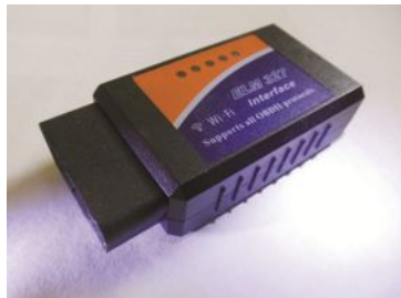
FIGURE 18.7 A Bluetooth adapter that plugs into the DLC and transmits global OBD-II information to a smart phone that has a scan tool app installed.
