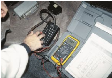
FIGURE 18.5 A breakout box is being used to diagnose an ABS problem.
