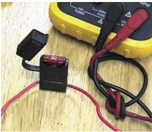
FIGURE 8-34 Note the blade-type fuse holder soldered in series with one of the meter leads. A 10-ampere fuse helps protect the internal meter fuse (if equipped) and the meter itself from damage that may result from excessive current flow if accidentally used incorrectly.
