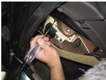
FIGURE 8-26 Testing a fuse with a test light. If the fuse is good, the test light should light on both sides (power side and load side) of the fuse.
