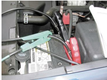
FIGURE 8-35 An inductive ammeter clamp is used with all starting and charging testers to measure the current flow through the battery cables.
