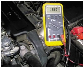
FIGURE 8-14 This digital multimeter set to read DC volts is being used to test the voltage of a vehicle battery. Most multimeters can also measure resistance (ohms) and current flow (amperes).
