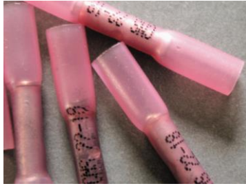
FIGURE 8-45 A typical crimp-and-seal connector. This type of connector is first lightly crimped to retain the ends of the wires and then it is heated. The tubing shrinks around the wire splice, and thermoplastic glue melts on the inside to provide an effective weather-resistant seal.
