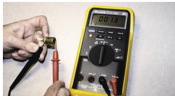
FIGURE 8-31 Using a digital multimeter set to read ohms ( \Omega ) to test this light bulb. The meter reads the resistance of the filament.
