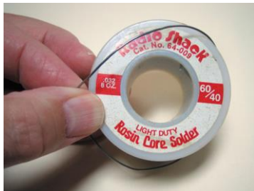
FIGURE 8-41 Always use rosin-core solder for electrical or electronic soldering. Also, use small-diameter solder for small soldering irons. Use large-diameter solder only for large-diameter (large-gauge) wire and higher-wattage soldering irons (guns).
