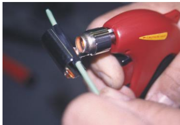
FIGURE 8-44 A butane torch especially designed for use on heat shrink applies heat without an open flame, which could cause damage.
