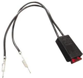
FIGURE 8-25 A technician-made fused jumper lead, which is equipped with a red 10-ampere fuse. This fused jumper wire uses terminals for testing circuits at a connector instead of alligator clips.
