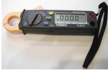
FIGURE 8-36 A typical mini clamp-on-type digital multimeter. This meter is capable of measuring alternating current (AC) and direct current (DC) without requiring that the circuit be disconnected to install the meter in series. The jaws are simply placed over the wire and current flow through the circuit is displayed.
