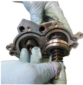
FIGURE 7-23 A band accumulator piston and spring being removed from a GM 4T65-E.
