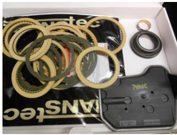
FIGURE 7-5 Most clutches included in overhaul kits use paper as the basis for the lining material.
