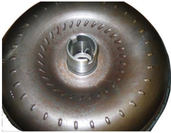
FIGURE 5-15 Visually check the pump drive notches or tangs for damage and the hub sealing surface for wear.
