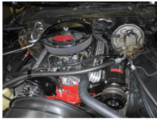
1 A restored 1971 Chevrolet Camaro has an aftermarket high-lift camshaft and does not idle correctly in drive with the stock torque converter.
