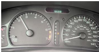
FIGURE 5-14 This 4-cylinder General Motors vehicle has a stall speed of about 2350 RPM. Notice that the gear selector is in drive and the speedometer is reading zero.
