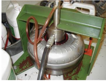
FIGURE 5-18 A leak-test fixture has been placed on the torque converter. It will be filled with ATF and then inspected for leaks.
