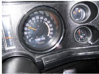
2 The stall speed of the stock torque converter was tested at 1850 RPM, which is normal for a stock engine but not for an engine equipped with a high-performance camshaft.
