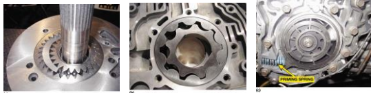
FIGURE 3-4 (a) Gear-type pump. (b) Gerotor-type pump. (c) Vane-type pump.
