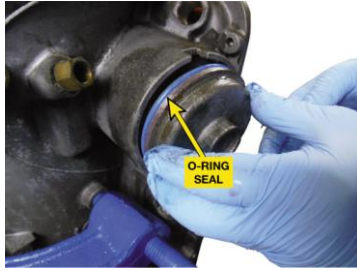
FIGURE 3-21 A new O-ring seal being installed on a cover.
