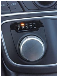
FIGURE 3-20 A rotary knob type electronic shifter used on a Chrysler 200.
