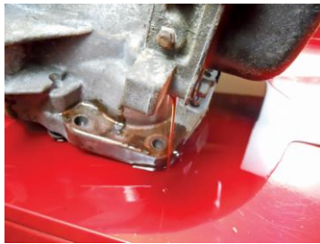
FIGURE 2-1 ATF being drained from a recycling center automatic transaxle still looks bright red in this unit being used for training.
