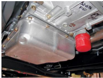
FIGURE 2-13 While most automatic transmissions use an internal filter only, this Allison transmission uses a spin-on-type filter that is designed to be replaced as part of routine service. There is another filter inside that is designed to be replaced only if the unit is overhauled or repaired.
