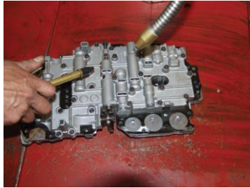
FIGURE 16-3 A valve body being washed and air dried in a parts washer. It will be cleaned again when the two major parts are separated.
