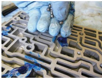
FIGURE 16-7 Using assembly lube is a great way to keep check balls in place during the reassembly of the valve body.
