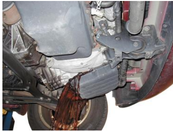
FIGURE 14-1 Draining the fluid from an automatic transaxle by allowing the fluid to flow into a container after most of the retaining bolts have been removed.
