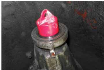
FIGURE 14-7 Using a plug helps prevent fluid loss when the driveshaft is removed.
