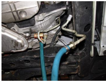
FIGURE 14-4 The lines from the fluid exchange machine can often be connected to the cooling lines from underneath the vehicle as on this front-wheel-drive General Motors vehicle.
