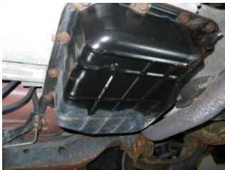
1 The owner of this Dodge pickup complained that automatic transmission fluid was leaking from the pan gasket.
