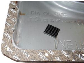
FIGURE 14-3 In this case, the cork-rubber gasket is glued to the pan and is ready to be installed. The retaining bolts need to be tightened in sequence, but be aware that over-tightening will cause a leak. Also, some manufacturers recommend using only an RTV sealer, but never use an RTV sealer and a gasket together.
