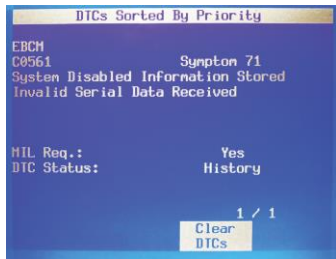
FIGURE 13-10 A “C” diagnostic trouble code was stored along with a note “symptom 71” which gives additional information about the possible cause of this serial data fault code being set.
