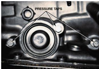
FIGURE 13–22 The locations (taps) for connecting a pressure gauge to measure the pressure of the various hydraulic circuits are usually found on the side of the automatic transmission/transaxle. Check service information for the exact locations for the vehicle being tested.
