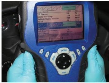
FIGURE 13–14 An OTC Genisys being used to troubleshoot a vehicle. This scan tool can be used on most makes and models of vehicles and is capable of diagnosing other computer systems in the vehicles such as automatic transmissions.
