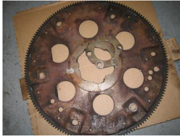
FIGURE 13-18 A broken flexplate that made a lot of noise and then the engine would not crank when it finally broke.
