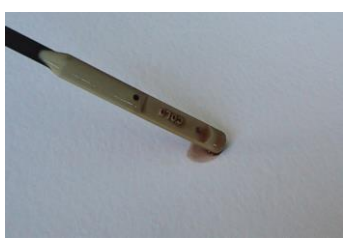
FIGURE 13-7 Fluid condition can be checked by placing a sample on clean, white, absorbent paper. Clean fluid will spread out and leave only a wet stain. Dirty fluid will leave deposits of foreign material.
