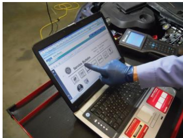
FIGURE 13-11 After checking for stored diagnostic trouble codes (DTCs), the wise technician checks service information for any technical service bulletins (TSBs) that may relate to the vehicle being serviced.
