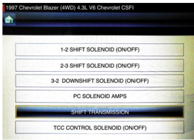
FIGURE 13-15 A Snap-on scan tool is able to shift the transmission and display pressure control (PC) solenoid current (amperes).
