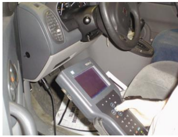
FIGURE 13–13 A TECH 2 scan tool is the factory scan tool used on General Motors vehicles.
