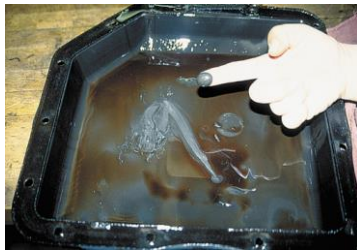
FIGURE 13-19 This is a normal amount of wear material in the bottom of an automatic transmission pan.
