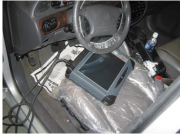
FIGURE 12-9 The use of a factory or a factory-level aftermarket scan tool is often needed to diagnose the dual clutch transmission system.
