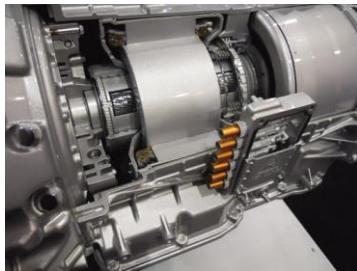
FIGURE 10-8 The two-mode transmission has orange high-voltage cables entering the unit to carry electric energy from the high-voltage battery pack to propel the vehicle and also to charge the battery during deceleration.
