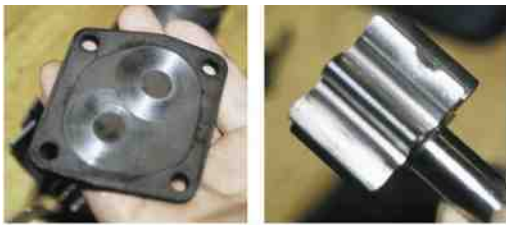
FIGURE 9-11 (a) A visual inspection indicated that this pump cover was worn. (b) An embedded particle of something was found on one of the gears, making this pump worthless except for scrap metal.
