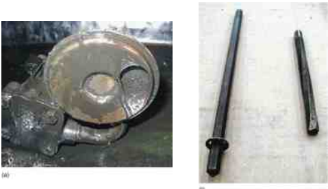
FIGURE 9-12 (a) The oil pump is the only part in an engine that gets unfiltered engine oil. The oil is drawn up from the bottom of the oil pan and is pressurized before flowing to the oil filter. (b) If debris gets into an oil pump, the drive or distributor shaft can twist and/or break. When this occurs, the engine will lose all oil pressure.
