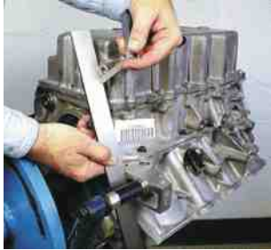
FIGURE 9-16 A straightedge and a feeler gauge are being used to check that the oil pan has been correctly installed on the 5.7-liter Chevrolet V-8 engine. The oil pan is part of the engine itself and must be properly installed to ensure that other parts attached to the engine are not being placed in a bind.
