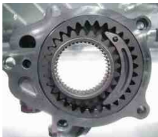
FIGURE 9-6 A typical oil pump mounted in the front cover of the engine that is driven by the crankshaft.
