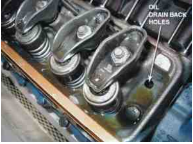
FIGURE 9-14 Oil is sent to the rocker arms on this Chevrolet V-8 engine through the hollow pushrods. The oil returns to the oil pan through the oil drainback holes in the cylinder head.
