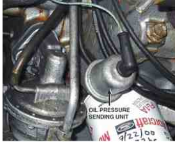
FIGURE 9-19 A typical oil pressure sending unit on a Ford V-8.
