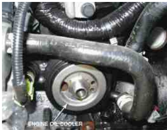
FIGURE 9-17 A typical engine oil cooler. Engine coolant flows through the cooler adjuster that fits between the engine block and the oil filter.
