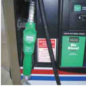
FIGURE 7-4 A pump decal indicating that the biodiesel fuel is ultra-low-sulfur diesel (ULSD) and must be used in 2007 and newer diesel vehicles.
