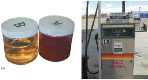
FIGURE 7-1 (a) Regular diesel fuel on the left has a clear or greenish tint, whereas fuel for off-road use is tinted red for identification. (b) A fuel pump in a farming area that clearly states the red diesel fuel is for off-road use only.
