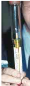
FIGURE 7-2 Testing the API viscosity of a diesel fuel sample using a hydrometer.
