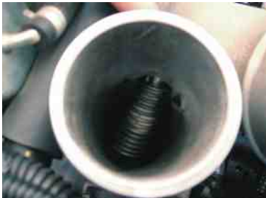
FIGURE 7-3 An electrical resistance heater coil in the air inlet on a General Motors 6.5-liter V-8 diesel engine used to warm the air entering the engine.
