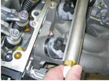
FIGURE 6-13 The fuel injectors used on this Honda Civic GX CNG engine are designed to flow gaseous fuel instead of liquid fuel and cannot be interchanged with any other type of injector.
