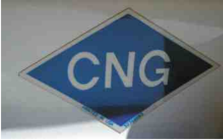
FIGURE 6-11 The blue sticker on the rear of this vehicle indicates that it is designed to use compressed natural gas.
