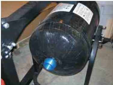
FIGURE 6-12 A CNG storage tank from a Honda Civic GX shown with the fixture used to support it while it is being removed or installed in the vehicle. Honda specifies that three technicians be used to remove or install the tank through the rear door of the vehicle due to the size and weight of the tank.
