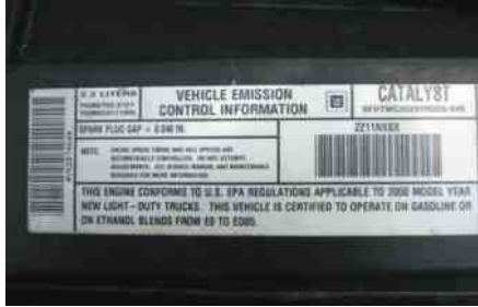
FIGURE 6-7 A vehicle emission control information (VECI) sticker on a flexible fuel vehicle indicating that it can use ethanol from 0 to 85%.
