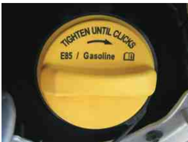
FIGURE 6-6 A flex-fuel vehicle often has a yellow gas cap, which is labeled E85/gasoline.
