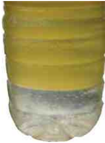
FIGURE 5-11 A container with gasoline containing alcohol. Notice the separation line where the alcohol-water mixture separated from the gasoline and sank to the bottom.
