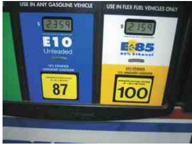
FIGURE 5-10 This fuel tank indicates that the gasoline is blended with 10% ethanol (ethyl alcohol) and can be used in any gasoline vehicle. E85 contains 85% ethanol and can only be used in vehicles specifically designed to use it.
