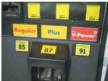
FIGURE 5-9 The posted octane rating in most high-altitude areas shows regular at 85 instead of the usual 87.
