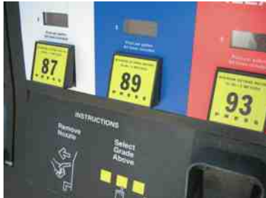
FIGURE 5-8 A pump showing regular with a pump octane of 87, plus rated at 89, and premium rated at 93. These ratings can vary with brand as well as in different parts of the country.
