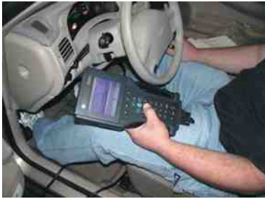
FIGURE 4-20 A scan tool is used to retrieve diagnostic trouble codes and to perform injector balance tests.
