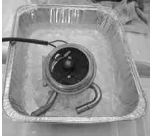
FIGURE 4-7 Using an ice bath to test the fuel temperature sensor.
