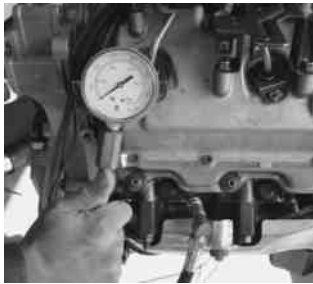
FIGURE 4-21 A compression gauge designed for the higher compression rate of a diesel engine should be used when checking the compression.
