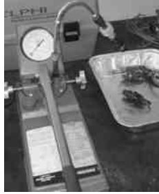
FIGURE 4-22 A typical pop tester used to check the spray pattern of a diesel engine injector.
