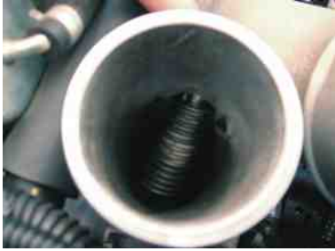
FIGURE 4-16 A wire wound electrical heater is used to warm the intake air on some diesel engines.
