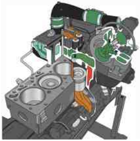
FIGURE 4-5 The common rail on a Cummins diesel engine. A high-pressure pump (up to 30,000 PSI) is used to supply diesel fuel to this common rail, which has tubes running to each injector. Note the thick cylinder walls and heavy-duty construction.
