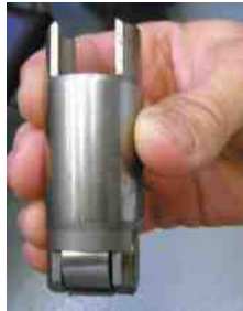
FIGURE 4-14 Roller lifter from a GM Duramax 6.6-liter V-8 diesel engine. Notice the size of this lifter compared to a roller lifter used in a gasoline engine.
