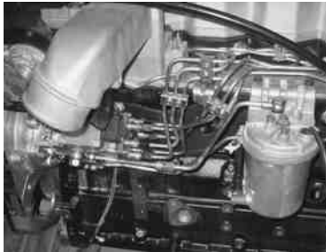
FIGURE 4-8 A typical distributor-type diesel injection pump showing the pump, lines, and fuel filter.
