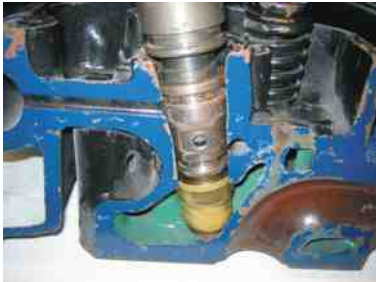
FIGURE 4-11 A HEUI injector from a Ford PowerStroke diesel engine. The grooves indicate the location of the O-rings.
