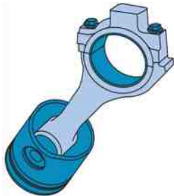
FIGURE 4-6 A rod/piston assembly from a 5.9-liter Cummins diesel engine used in a Dodge pickup truck.
