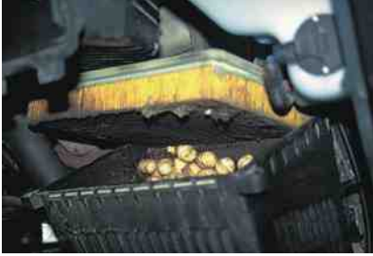
FIGURE 33-4 This is what was found when removing an air filter from a vehicle that had a lack-of-power concern. Obviously the nuts were deposited by squirrels or some other animal, blocking a lot of the airflow into the engine.
