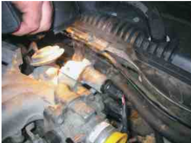
FIGURE 33-5 Using a bright light makes seeing where the smoke is coming from easier. In this case, smoke was added to the intake manifold with the inlet blocked with a yellow plastic cap and smoke was seen escaping past a gasket at the idle air control.
