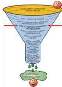
FIGURE 33-7 Step 3 in the diagnostic process is to retrieve any stored diagnostic trouble codes.
