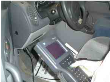
FIGURE 33-17 The first step in the reprogramming procedure is to determine the current software installed using a scan tool. Not all scan tools can be used. In most cases using the factory scan tool is needed for reprogramming unless the scan tool is equipped to handle reprogramming.
