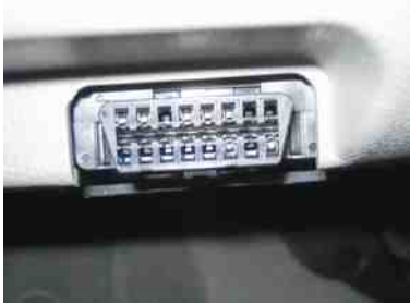
FIGURE 33-16 A typical OBD-II data link connector (DLC). The location varies with make and model and may even be covered, but a tool is not needed to gain access. Check service information for the exact location if needed.
