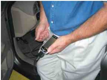
FIGURE 33–12 Some scan tools use pocket PCS which make it very convenient to use.
