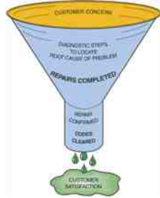
FIGURE 33-1 A funnel is one way to visualize the diagnostic process. The purpose is to narrow the possible causes of a concern until the root cause is determined and corrected.
