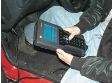
FIGURE 33–11 A TECH 2 scan tool is the factory scan tool used on General Motors vehicles.
