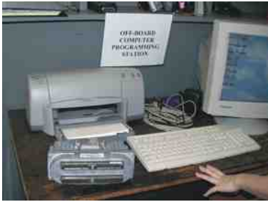
FIGURE 33-20 Connecting cables and a computer to perform off-board programming.
