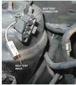
FIGURE 33-14 A Ford OBD-I self-test connector. The location of this connector can vary with model and year of vehicle.
