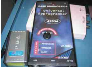
FIGURE 33-22 A typical J2534 universal reprogrammer that uses the J2534 standards.
