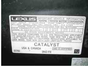
FIGURE 31-1 The underhood decal showing that this Lexus RX-330 meets both national (Tier 2, BIN 5) and California LEV-II (ULEV) regulation standards.
