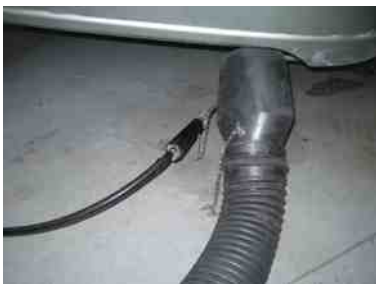
FIGURE 31-6 A partial stream sampling exhaust probe being used to measure exhaust gases in parts per million (PPM) or percent (%).
