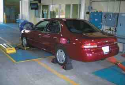
FIGURE 31-4 A vehicle being tested during an enhanced emission test.
