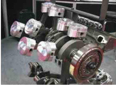
FIGURE 3-1 The rotating assembly for a V-8 engine that has eight pistons and connecting rods and one crankshaft.
