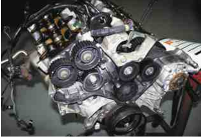
FIGURE 3-13 A dual overhead camshaft (DOHC) V-8 engine with the cam cover removed.
