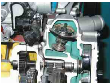
FIGURE 3-3 The coolant temperature is controlled by the thermostat which opens and allows coolant to flow to the radiator when the temperature reaches the rating temperature of the thermostat.
