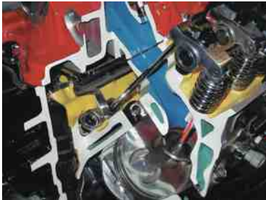
FIGURE 3-11 Cutaway of a V-8 engine showing the lifters, pushrods, roller rocker arms, and valves.
