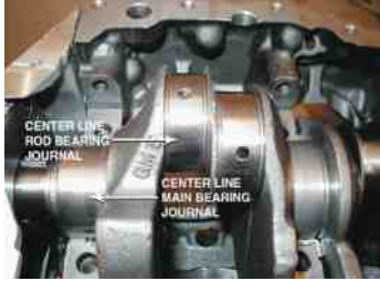
FIGURE 3-19 The distance between the centerline of the main bearing journal and the centerline of the connecting rod journal determines the stroke of the engine. This photo is a little unusual because this is from a V-6 with a splayed crankshaft used to even out the impulses on a 90° V-6 engine design.
