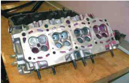
FIGURE 3-2 A cylinder head with four valves per cylinder, two intake valves (larger) and two exhaust valves (smaller) per cylinder.
