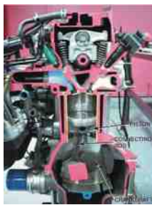
FIGURE 3-6 Cutaway of an engine showing the cylinder, piston, connecting rod, and crankshaft.
