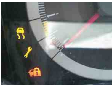
FIGURE 29-9 A wrench symbol warning lamp on a Ford vehicle. The symbol can also be green.
