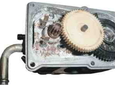
FIGURE 29-12 A corroded electronic throttle control assembly shown with the cover removed.
