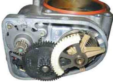
FIGURE 29-13 Notice the small motor gear on the left drives a larger plastic gear (black), which then drives the small gear in mesh with the section of a gear attached to the throttle plate. This results in a huge torque increase from the small motor and helps explain why it could be dangerous to insert a finger into the throttle body assembly.
