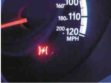
FIGURE 29-10 A symbol used on a Chrysler vehicle indicating a fault with the electronic throttle control.
