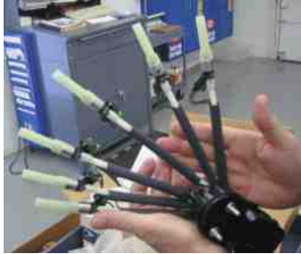
FIGURE 27-19 A factory replacement unit for a CSFI unit that has individual injectors at the ends that go into the intake manifold instead of poppet valves.
