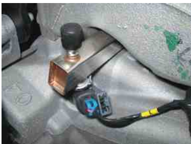
FIGURE 27-15 A rectangular-shaped fuel rail is used to help dampen fuel system pulsations and noise caused by the injectors opening and closing.
