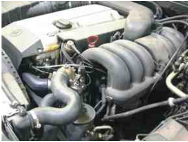
FIGURE 27-8 A port fuel-injected engine that is equipped with long, tuned intake manifold runners.
