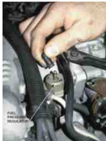
FIGURE 26-24 If the vacuum hose is removed from the fuel-pressure regulator when the engine is running, the fuel pressure should increase. If it does not increase, then the fuel pump is not capable of supplying adequate pressure or the fuel-pressure regulator is defective. If gasoline is visible in the vacuum hose, the regulator is leaking and should be replaced.
