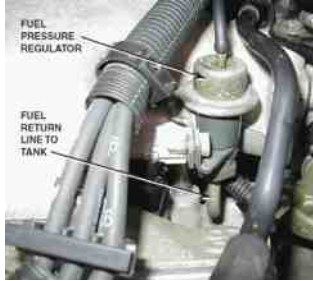
FIGURE 26-25 Fuel should be heard returning to the fuel tank at the fuel return line if the fuel pump and fuel-pressure regulator are functioning correctly.
