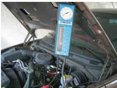
FIGURE 26-27 A fuel system tester connected in series in the fuel system so all of the fuel used flows through the meter which displays the rate-of-flow and the fuel pressure.
