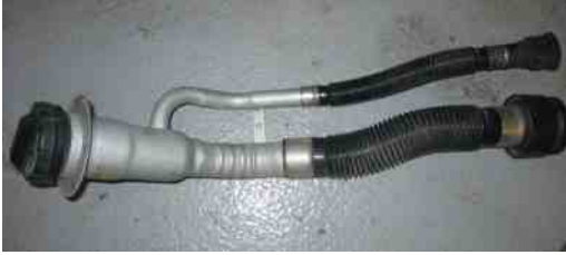
FIGURE 26-4 Vehicles equipped with onboard refueling vapor recovery usually have a reduced-size fill tube.
