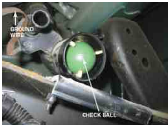
FIGURE 26-3 A view of a typical filler tube with the fuel tank removed. Notice the ground strap used to help prevent the buildup of static electricity as the fuel flows into the plastic tank. The check ball looks exactly like a ping-pong ball.
