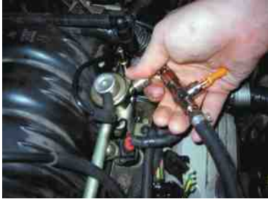
FIGURE 26-22 The Schrader valve on this General Motors 3800 V-6 is located next to the fuel-pressure regulator.
