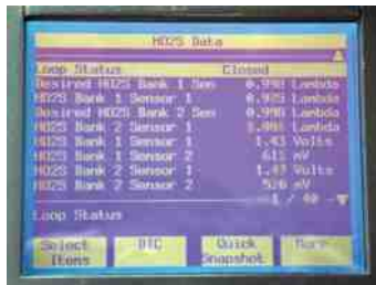
FIGURE 24-26 The target lambda on this vehicle is slightly lower than 1.0 indicating that the PCM is attempting to supply the engine with an air-fuel mixture that is slightly richer than stoichiometric. Multiply the lambda number by 14.7 to find the actual air-fuel ratio.
