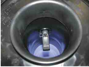
FIGURE 23-4 The sensing wire in a typical hot wire mass air flow sensor.
