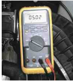
FIGURE 21-5 Checking the 5-volt reference from the computer being applied to the TP sensor with the ignition switch on (engine off).
