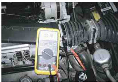
FIGURE 21-6 Checking the voltage drop between the TP sensor ground and a good engine ground with the ignition on (engine off). A reading of greater than 0.2 volt (200 mV) represents a bad computer ground.
