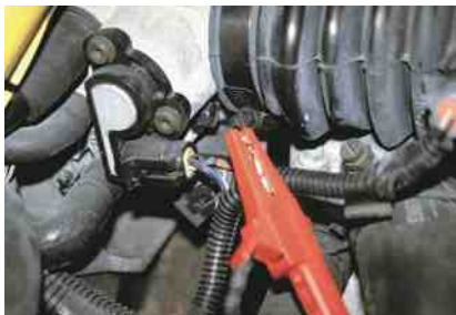
FIGURE 21-3 A meter lead connected to a T-pin that was gently pushed along the signal wire of the TP sensor until the point of the pin touched the metal terminal inside the plastic connector.
