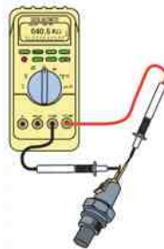
FIGURE 20-5 Measuring the resistance of the ECT sensor. The resistance measurement can then be compared with specifications. (Courtesy of Fluke Corporation)
