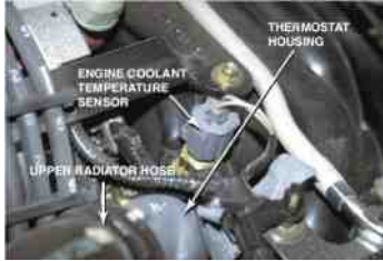
FIGURE 20-1 A typical engine coolant temperature (ECT) sensor. ECT sensors are located near the thermostat housing on most engines.
