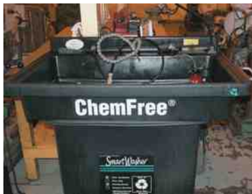
FIGURE 2-6 Using a water-based cleaning system helps reduce the hazards from using strong chemicals.
