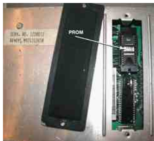
FIGURE 18-3 A replaceable PROM used in an older General Motors computer. Notice that the sealed access panel has been removed to gain access.
