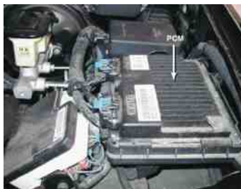
FIGURE 18-12 This Powertrain Control Module (PCM) is located under the hood on this Chevrolet pickup truck.
