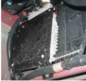
FIGURE 18-13 This PCM on a Chrysler vehicle can only be seen by hoisting the vehicle because it is located next to the radiator, and in the airflow to help keep it cool.
