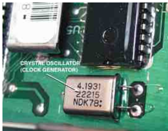
FIGURE 18-11 The clock generator produces a series of pulses that are used by the microprocessor and other components to stay in step with each other at a steady rate.
