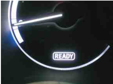
FIGURE 14-8 A Toyota/Lexus hybrid electric vehicle has a ready light. If the ready light is on, the engine can start at anytime without warming.
