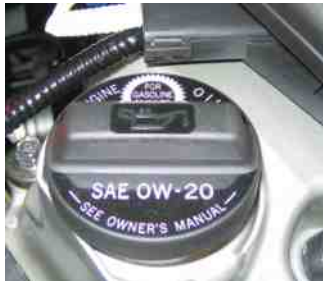
FIGURE 14-9 Always use the viscosity of oil as specified on the oil fill cap.
