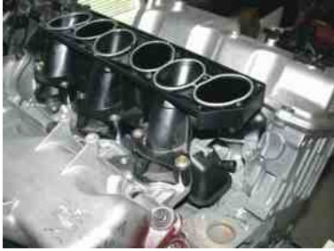
FIGURE 14-4 The lower intake manifold, attaches to the cylinder heads.
