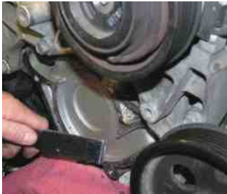
FIGURE 14-2 Use caution if using a steel scraper to remove a gasket from aluminum parts. It is best to use a wood or plastic scraper.
