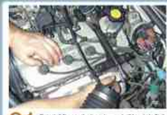
21 Reinsert the spark plug wires and all brackets that were removed to gain access to the valve cover.
