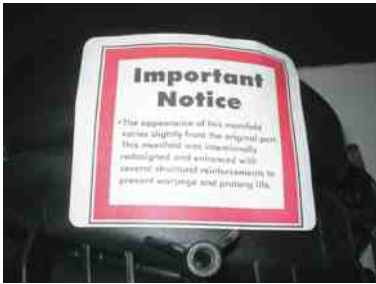
FIGURE 14-6 Many aftermarket replacement intake manifolds have a different appearance from the original manifold.
