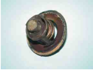
FIGURE 14-1 A stuck-open thermostat. This caused the vehicle to set a diagnostic trouble code P0128 (coolant temperature below thermostat regulating temperature).
