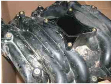
FIGURE 14-5 The upper intake manifold, often called a plenum, attaches to the lower intake manifold.
