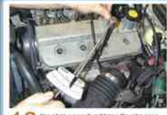
19 Use a torque wrench and torque the valve cover retaining bolts to factory specifications.
