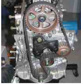
FIGURE 14-7 A single overhead camshaft engine with a timing belt that also rotates the water pump.
