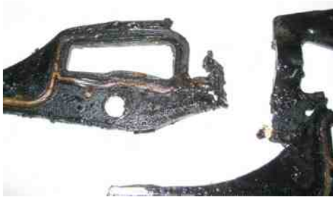
FIGURE 14-3 An intake manifold gasket that failed and allowed coolant to be drawn into the cylinder(s).
