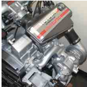
FIGURE 12-2 A turbocharger on a Toyota engine.
