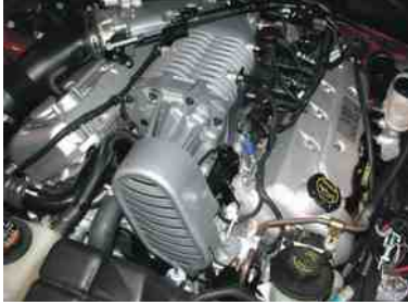
FIGURE 12-1 A supercharger on a Ford V-8.
