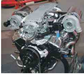
FIGURE 12-13 A dual turbocharger system installed on a small block Chevrolet V-8 engine.
