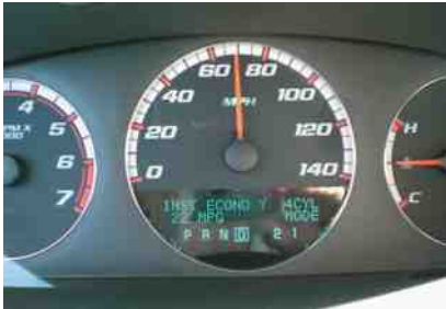
FIGURE 11-17 The driver information display on a Chevrolet Impala with a 5.3 liter V-8 equipped with active fuel management. The transition between 4-cylinder mode and 8-cylinder mode is so smooth that most drivers are not aware that the switch is occurring.
