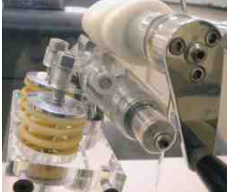
FIGURE 11-10 A plastic mock-up of a Honda VTEC system that uses two different camshaft profiles, one for low-speed engine operation and the other for high speed.
