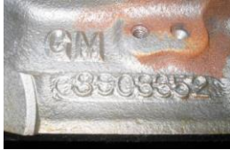
FIGURE 9-5 Engine block identification number cast into the block is used for identification.
