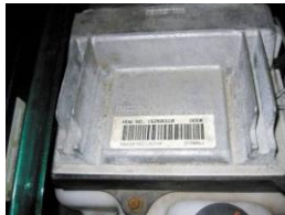
FIGURE 9-4 A typical computer calibration sticker on the case of the controller. The information on the sticker is often needed when ordering parts or a replacement controller.
