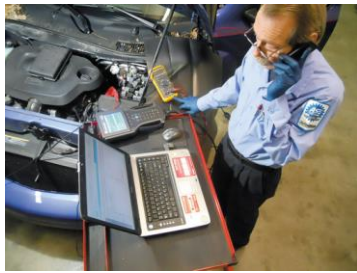
FIGURE 8-4 Whenever calling a hot line service be sure that you have all of the vehicle information ready and are prepared to give answers regarding voltage readings or scan tool data when talking to the vehicle specialist.
