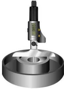
FIGURE 7-21 A digital readout depth micrometer.
