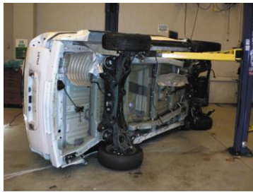
FIGURE 6-5 This training vehicle fell from the hoist when the pads were not set correctly. No one was hurt, but the vehicle was damaged.
