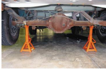
FIGURE 6-2 Safety stands are being used to support the rear of this vehicle.
