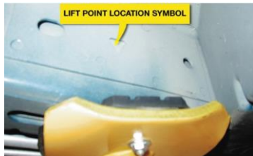
FIGURE 6-3 Most newer vehicles have a triangle symbol indicating the recommended hoisting lift points.
