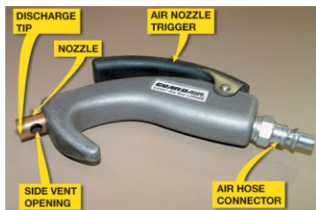
FIGURE 5-2 Always use an air nozzle that is OSHA approved. The openings in the side are used to allow air to escape if the nozzle tip were to become clogged.
