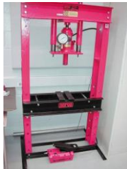
FIGURE 5-12 A hydraulic press is usually used to press bearings on and off of rear axles and transmissions.
