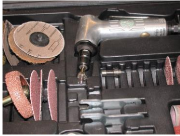
FIGURE 5-8 This typical die grinder surface preparation kit includes the air-operated die grinder, as well as a variety of sanding discs for smoothing surfaces or removing rust.
