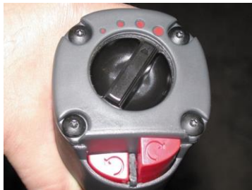
FIGURE 5-4 This impact wrench features a variable torque setting using a rotary knob. The direction of rotation can be changed by pressing the button at the bottom.
