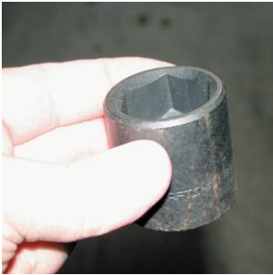
FIGURE 5-6 A black impact socket. Always use impact-type sockets whenever using an impact wrench to avoid the possibility of shattering the socket, which can cause personal injury.
