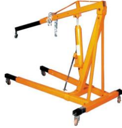
FIGURE 5-13 A typical portable crane used to lift and move heavy assemblies, such as engines and transmissions.
