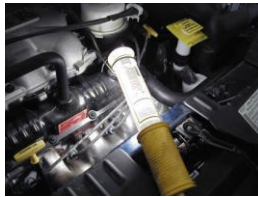
FIGURE 5-9 A fluorescent trouble light operates cooler and is safer to use in the shop because it is protected against accidental breakage where gasoline or other flammable liquids would happen to come in contact with the light.
