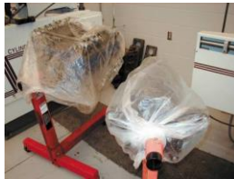
FIGURE 5-14 Two engines on engine stands. The plastic bags over the engines help keep dirt from getting onto these engines and engine parts.
