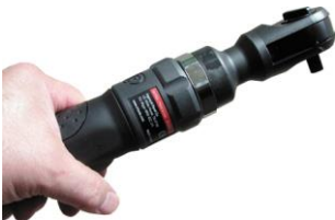
FIGURE 5-7 An air ratchet is a very useful tool that allows fast removal and installation of fasteners, especially in areas that are difficult to reach or do not have room enough to move a hand ratchet wrench.
