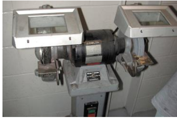
FIGURE 5-10 A typical pedestal grinder with a wire wheel on the left side and a stone wheel on the right side. Even though this machine is equipped with guards, safety glasses or a face shield should always be worn when using a grinder or wire wheel.
