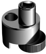
FIGURE 4-37 A stud remover uses an offset serrated wheel to grasp the stud so it will be rotated when a ratchet or breaker bar is used to rotate the assembly.
