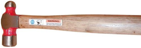
FIGURE 4-21 A typical ball-peen hammer.
