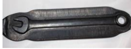
FIGURE 4-1 A forged wrench after it has been forged but before the flashing, extra material around the wrench, has been removed.
