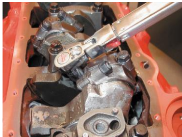
FIGURE 4-13 Using a torque wrench to tighten connecting rod nuts on an engine.
