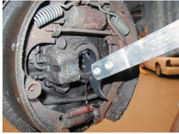
FIGURE 4-44 A seal puller being used to remove a seal from a rear axle.
