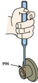
FIGURE 4-34 A punch used to drive pins from assembled components. This type of punch is also called a pin punch.
