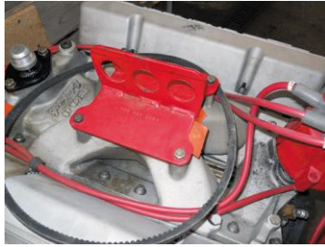
FIGURE 35-6 A fixture installed that is used as a place to attach the hosting chains.
