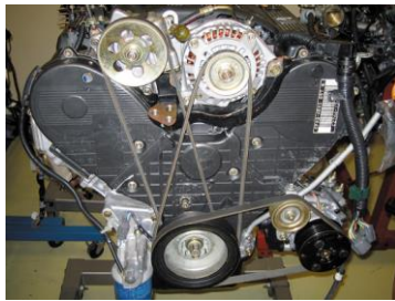
FIGURE 35-5 It is often easier to install all of the accessory drive belts before the engine is installed in the vehicle.
