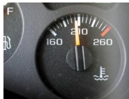
FIGURE 35-7 Even though the dash gauge may show normal operating temperature, a scan tool or an infrared pyrometer can also be used to verify proper coolant temperature.
