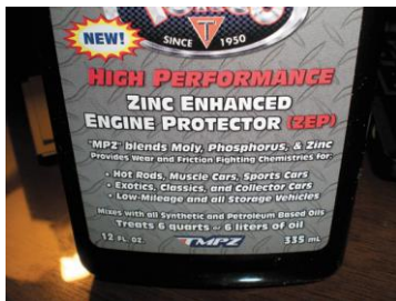
FIGURE 34-27 A commercial additive designed to protect a flat-bottom lifter camshaft used in older vehicles when using newer oils that do not have enough ZDDP to protect the camshaft and lifters.
