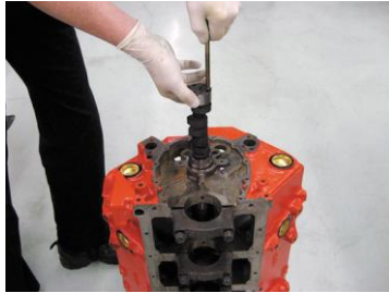
FIGURE 34-26 Installing a camshaft is easier if the engine is vertical so gravity can help, and this method reduces the possibility of damaging the cam bearings.
