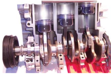
FIGURE 34-1 A Ford 1.0 liter 3-cylinder engine is different than many small engines and may require detailed service information to be sure that all of the steps are taken for proper assembly.
