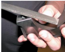
FIGURE 34-2 Deburring all sharp edges is an important step to achieve proper engine assembly.
