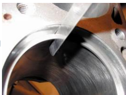
FIGURE 34-28 A feeler gauge is used to check piston ring gap.
