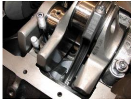
FIGURE 34-8 A trial assembly showed that some grinding of the block will be needed to provide clearance for the counterweight of the crankshaft. Also, notice that the engine has been equipped with studs for the four-bolt
