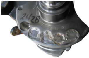
FIGURE 33-6 Heavy metal installed and welded in place.
