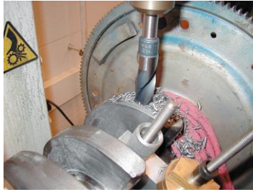
FIGURE 33-5 A drill is often used to remove weight from the crankshaft to achieve proper balance.
