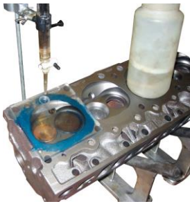
FIGURE 33-7 Setup needed to measure the combustion chamber volume in cubic centimeters (cc).
