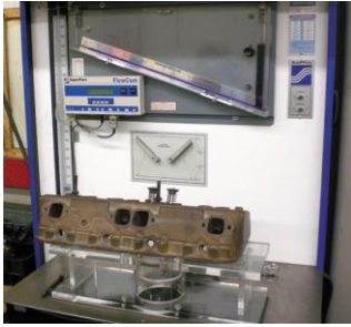
FIGURE 33-10 A flow bench that can measure and record the airflow through the intake and exhaust ports of each cylinder.
