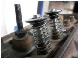
FIGURE 33-8 Cylinder head setup for flow testing. Note the weak valve springs that are strong enough to keep the valves shut, yet weak enough to permit the flow bench operator to vary the intake valve opening amount.
