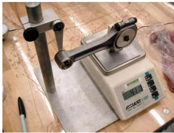
FIGURE 33-1 Weighing the big end of a connecting rod on a scale that keeps it perfectly horizontal so that each end can be weighed separately.
