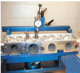
FIGURE 33-9 Modeling clay is installed around the port to duplicate the flow improvement characteristics of an intake manifold.
