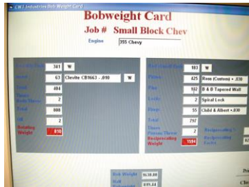
FIGURE 33-4 The display of a crankshaft balancer showing where weight needs to be removed to achieve a balanced assembly.
