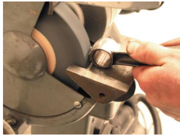
FIGURE 33-2 Removing material from the balancing pad on the small end of the rod to match it to the weight of the small end of the lightest rod being used in the engine.
