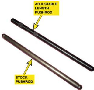
FIGURE 33-17 An adjustable pushrod is adjustable for length compared to a conventional stock pushrod.
