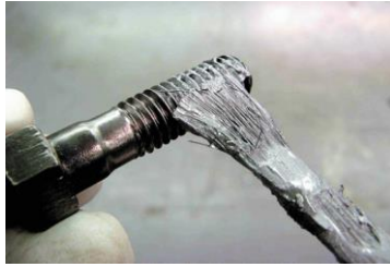
FIGURE 32-16 Applying antiseize compound to the threads of a bolt helps prevent the threads from galling or rusting.
