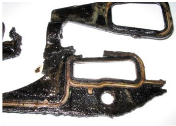
FIGURE 32-11 This intake manifold gasket was damaged due to fretting. Newer designs allow for more movement between the intake manifold and the cylinder head.
