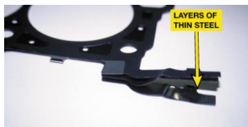
FIGURE 32-6 Multilayer steel (MLS) gaskets are used on many newer all-aluminum engines as well as on engines that use a cast block with aluminum cylinder heads. This type of gasket allows the aluminum to expand without losing the sealing ability of the gasket.
