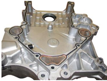
FIGURE 32-9 Formed in place gaskets often use silicone rubber and are applied at the factory using a robot. Check gasket manufacturers for the correct gasket replacement.
