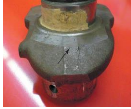
FIGURE 31-5 Wide separation lines of a forged crankshaft.
