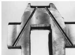
FIGURE 31-8 Crankshaft sawed in half, showing drilled oil passages between the main and rod bearing journals.
