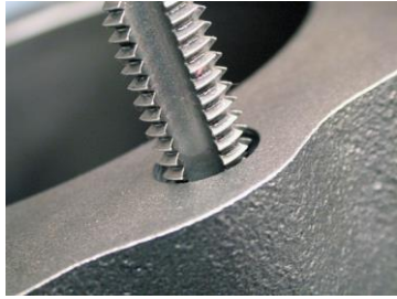
FIGURE 30–35 A tread chaser or bottoming tap should be used in all threaded holes before assembling the engine.
