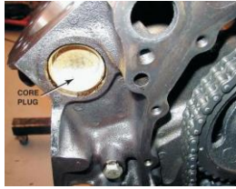
FIGURE 30-2 An expansion (core) plug is used to block the opening in the cylinder head or block the holes where the core sand was removed after the part was cast.
